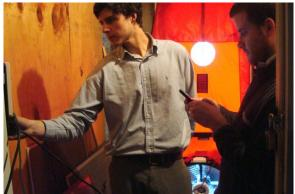
An energy auditor with the Energy Savers team conducts a blower door test to check for air leakage.
