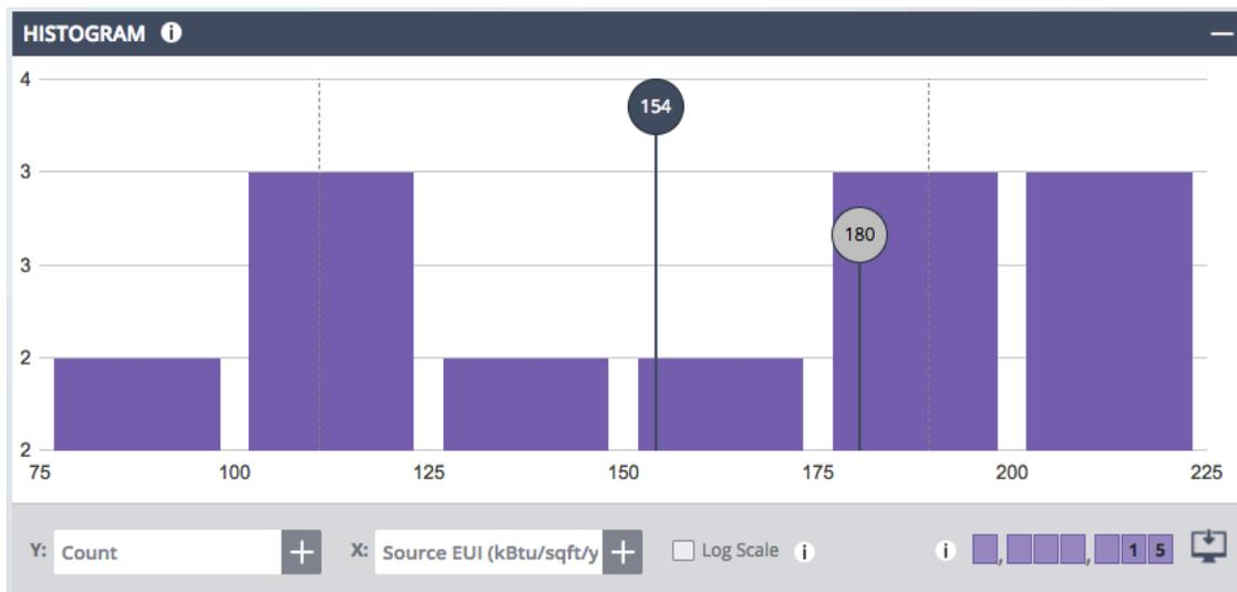
Figure 19. Screen image from the DOE Building Performance Database (BPD) showing measured source EUI distribution for a peer group of 15 hotels in climate zone 5B (cool-dry), less than 100,000 sf. Grey balloon shows source EUI for simulated building.
