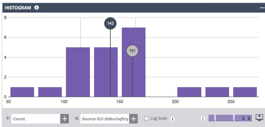
Figure 14. Screen image from the DOE Building Performance Database (BPD) showing measured source EUI distribution for a peer group of 22 office buildings in San Jose, ranging in size from 50,000-90,000 sf. Grey balloon shows source EUI for simulated building.
