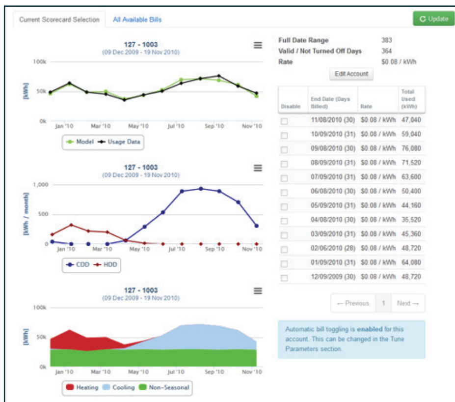
Figure 28: Weather-Based Regression and Energy End Use Separation (EnergyScoreCards, sample electric account)
