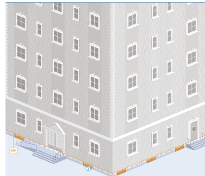
1 Engineered flood vents allow water to infiltrate non-living space.
